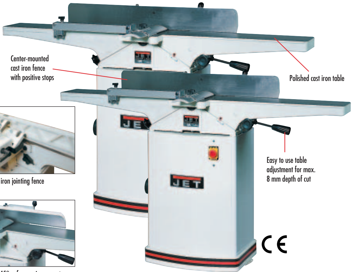
Jointing fence tilts \pm 45^\circ – for maximum protection, also when cutting chamfers
